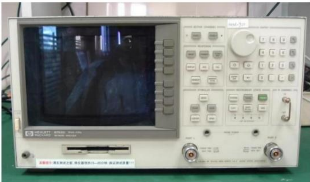
Antenna Measuring Network Analyzer
